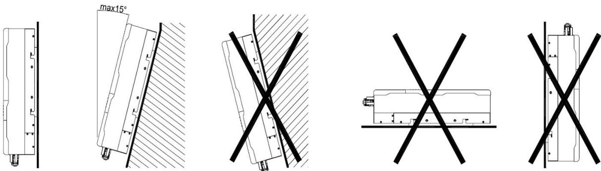
Fig.3 Recommended installed position of the inverter
