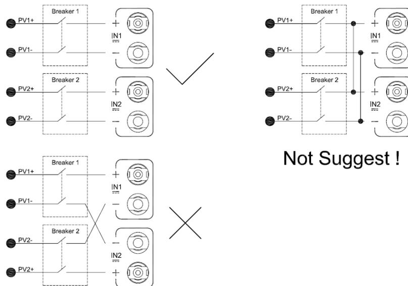
**Note:** Ensure that photovoltaic field voltage polarity matches the “+” and “-” symbols. Before connecting the IGSI “DJ” series inverters with the photovoltaic field, it is recommended to check, using a proper gauge, that the polarity value and the voltage allowed value between positive and negative contacts are correct.
