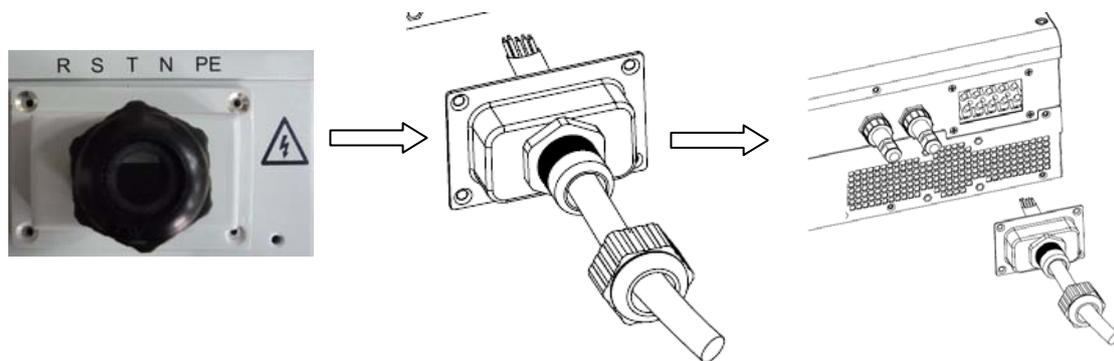
Fig. 10 AC terminals under AC terminals cover
