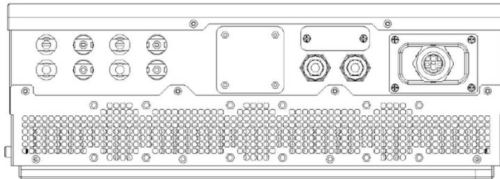
Fig. 9 Connections on the bottom of the inverter
