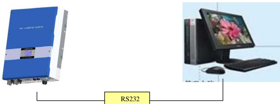
**NOTE:** Please use only the special RS232 cable. If the length is not insufficient, extend it using the “extended RS232 cable” from the local market.
