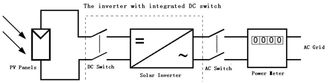
Fig.8 The PV system diagram 2
