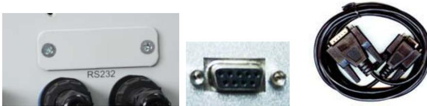
Fig. 10 RS232 serial port and special RS232 cable
