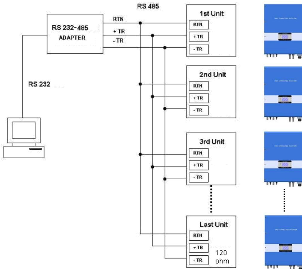
Fig.12 Multiple daisy-chain connection
