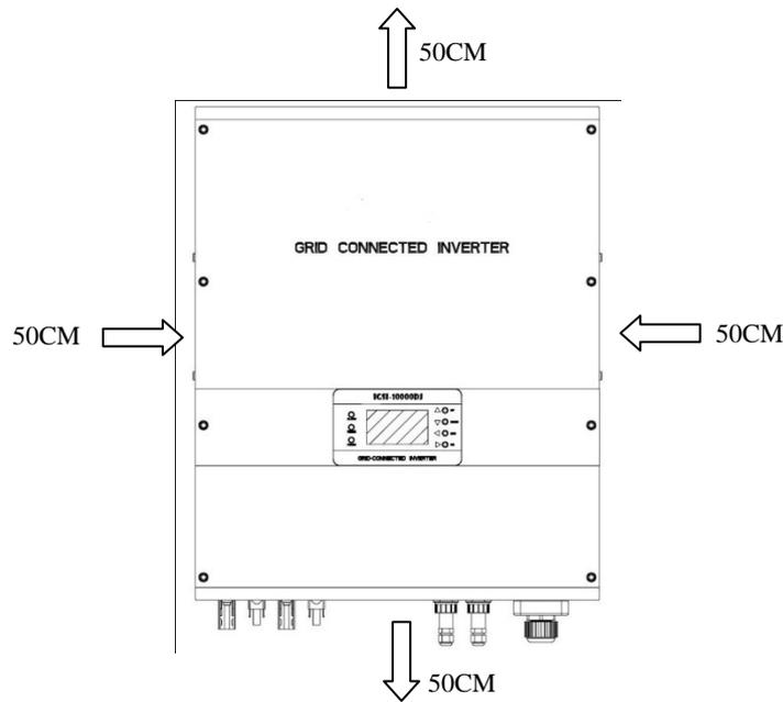
Fig.2 Minimum clearance around inverter
